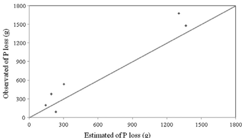
Fig. 3. Relationship between estimated and observed P losses using the C-MUSLE model.
