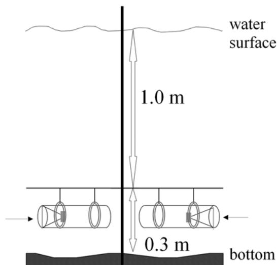
Fig. 1. Diagram of traps used for collecting YOY perch.
